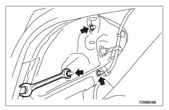
2. Remove the light case mounting nuts. Disconnect the connector.
